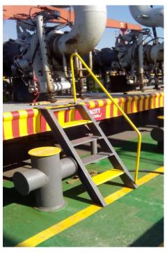
All the portable stairs, ramps or other fittings made available shall be arranged to be properly secured to the manifold platform edge.
